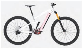
Positioning of the Bosch PowerTube battery as close as possible to the motor thanks to the Moustache fixings.
