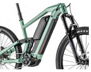
To equipe our new Weekend with the Bosch DualBattery technology, we have worked on the frame by replacing the top tube with a new version, offering the necessary space to house 500Wh more.
