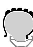
Figure 29. Inner tube in the rim
