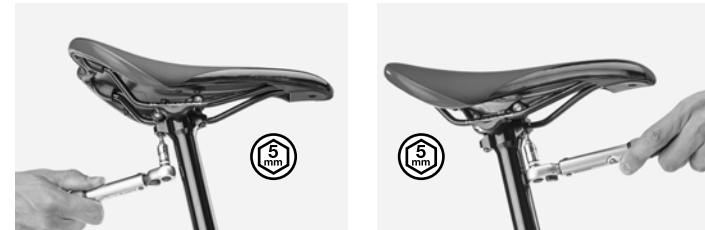
Figure 9. Steps for tightening/loosening the fitting blocks.
