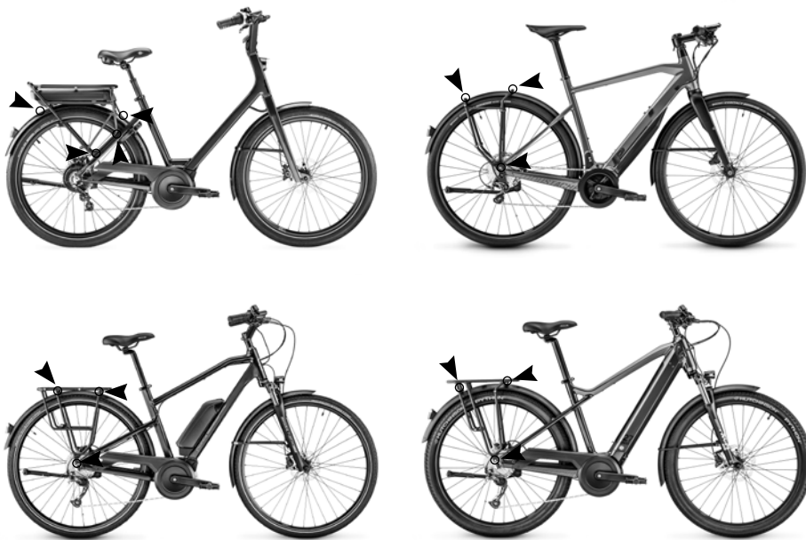
Figure 35. Luggage's fixing points represented by the black arrows.
