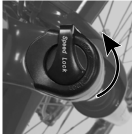
Figure 19. Locking lever in open position.
