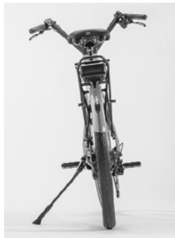
Figure 31. Ideal angle on flat ground.
