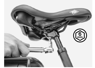
Figure 8. Tightening/loosening the fitting block.
