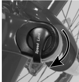
Figure 20. Locking lever in close position.
