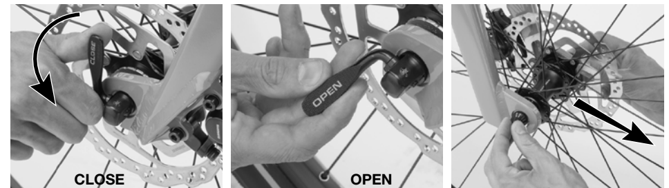
Figure 15. Opening the quick release axle.
