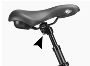
Figure 6. Saddle with one fitting block.
