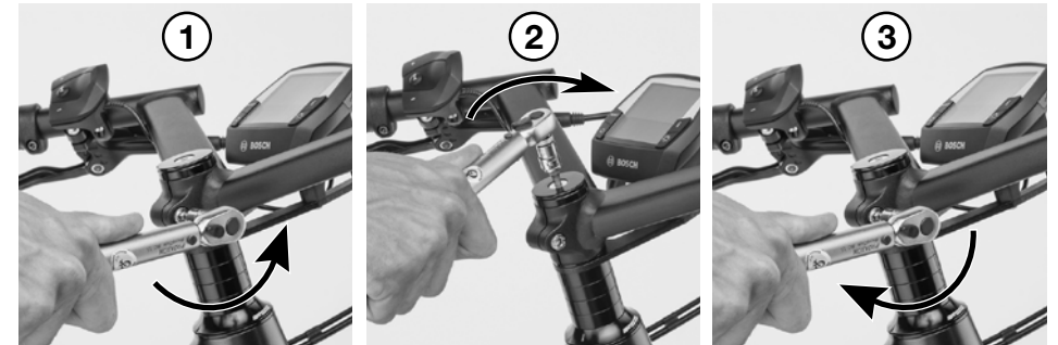
Figure 12. Stages for the headset settings.
