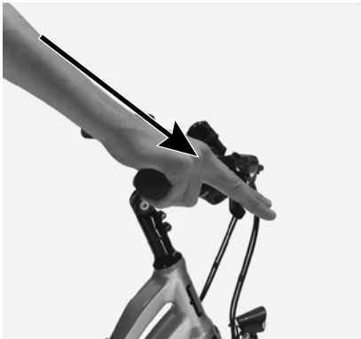
Figure 10. Brake lever aligned with the forearm.
