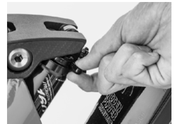
Figure 23. Manipulating the valve cap.
