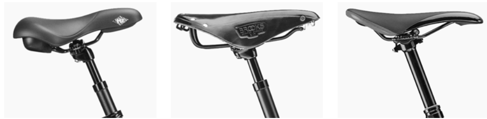
Figure 5. Saddle angle settings for Monday 26 (left), mixed use (middle) and MTB use (right).
